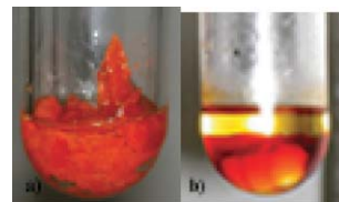
Fig. 1 (a) Mesitylene and [Hmim][Br 3 ] at room temperature (1:1 molar ratio); (b) reaction mixture at 70 °C, after 24 h (the upper phase constitutes the product).
